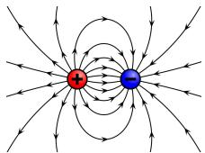
Electric field diagrams show the direction of electric force on a positive test charge.
