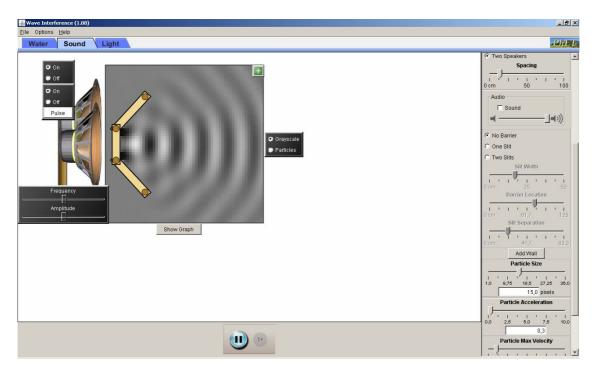
*Figure 2. High frequency radiation pattern of a real cone speaker simulated with two point source*
